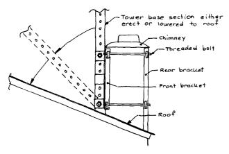
fig. 5. Remove upper mast bolt to lower tower to roof.
